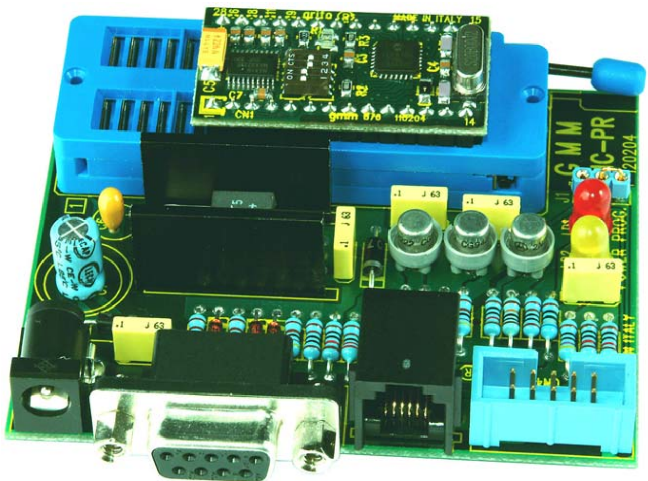
FIGURE 28: GMM PIC-PR PROGRAMMER WITH GMM 876 INSTALLED ON ZIF SOCKET
