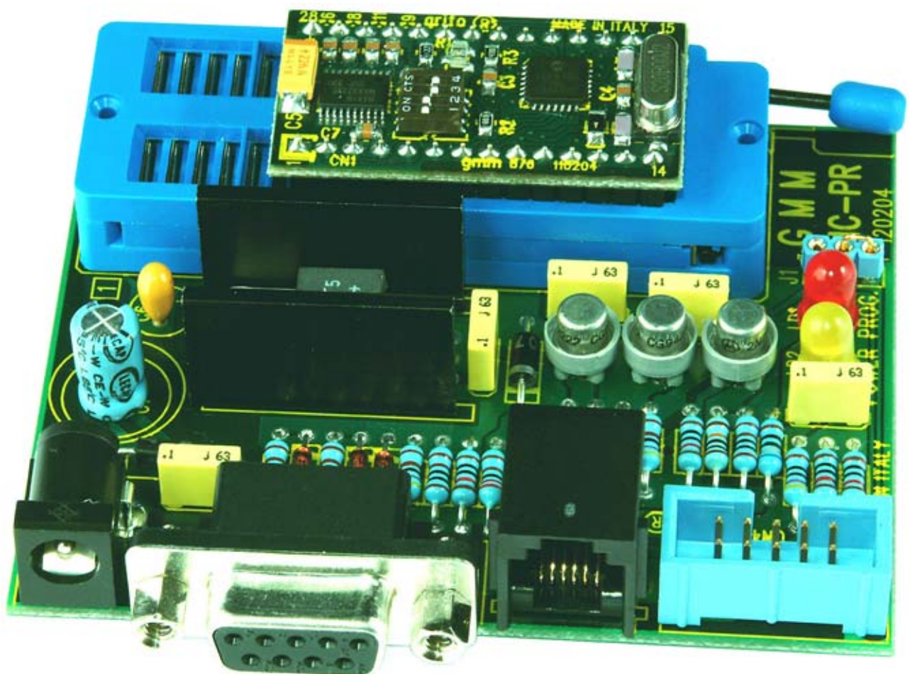
FIGURE 28: GMM PIC-PR PROGRAMMER WITH GMM 886 INSTALLED ON ZIF SOCKET
