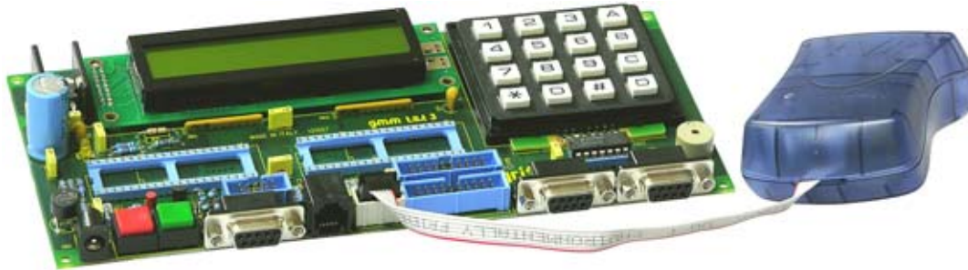
FIGURE D4: AVRISP MK II CONNECTED TO GMM TST3
