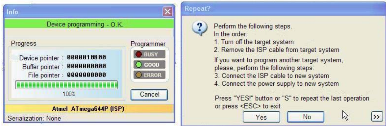
FIGURE D15: ISP PROGRAMMING WITH MP-AVR51/USB
