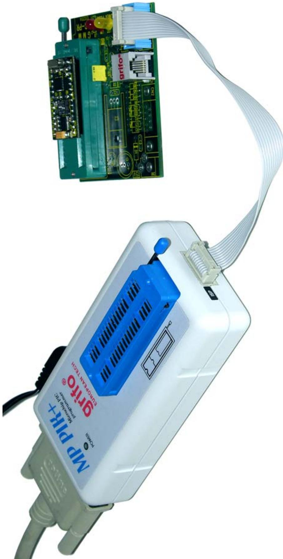
FIGURE 15: USING THE PROGRAMMER THROUGH MP PIK+
