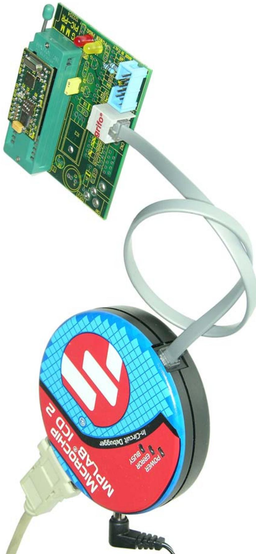
FIGURE 10: USING THE PROGRAMMER THROUGH MPLAB® ICD 2
