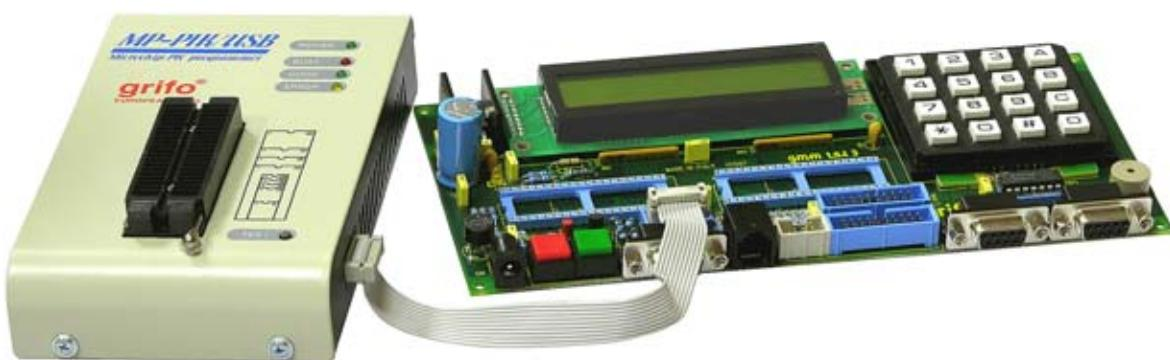
**FIGURE 27: LINK BETWEEN GMM TST 3 AND MP PIK/USB**
