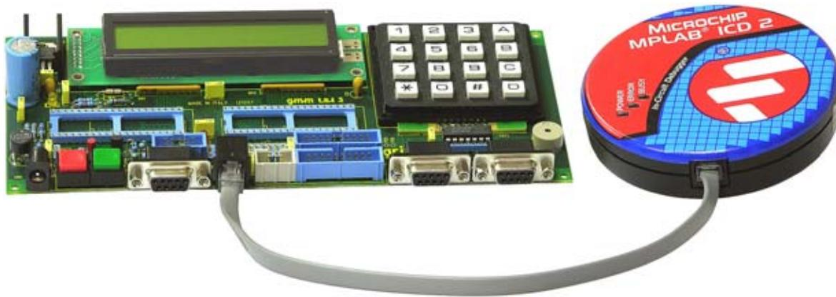
**FIGURE 25:** LINK BETWEEN GMM TST 3 AND MPLAB® ICD2
