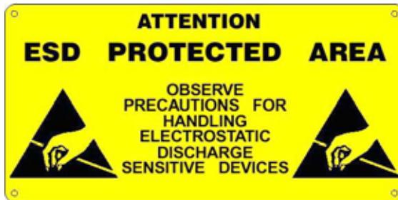
Pins of module are not provided with any kind of ESD protection. Many pins of the card are directly connected to their respective pins of on board's components and these last are sensitive to electrostatic noises. So personnel who handles the product/s is invited to take all necessary precautions that avoid possible damages caused by electrostatic discharges.
